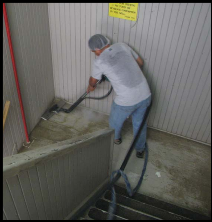
Using floor suction tool to clean landing of mustard and dirt “tar”. To speed cleaning, detergent is added in a parallel circuit with the steam. The suction capability removes the water, detergent and dissolved soils leaving the floor clean and dry.
