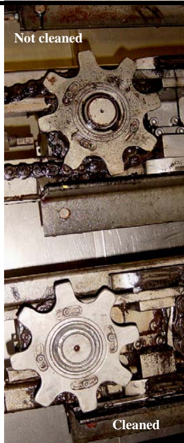
With the ability to add detergents and degreasers in a parallel circuit with the vapor, the equipment can quickly and easily remove greases and built up soils from equipment.
