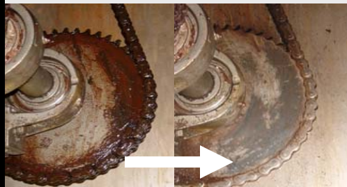
With the ability to add detergents and degreasers in a parallel circuit with the vapor, the equipment can quickly and easily remove greases and built up soils from equipment.
