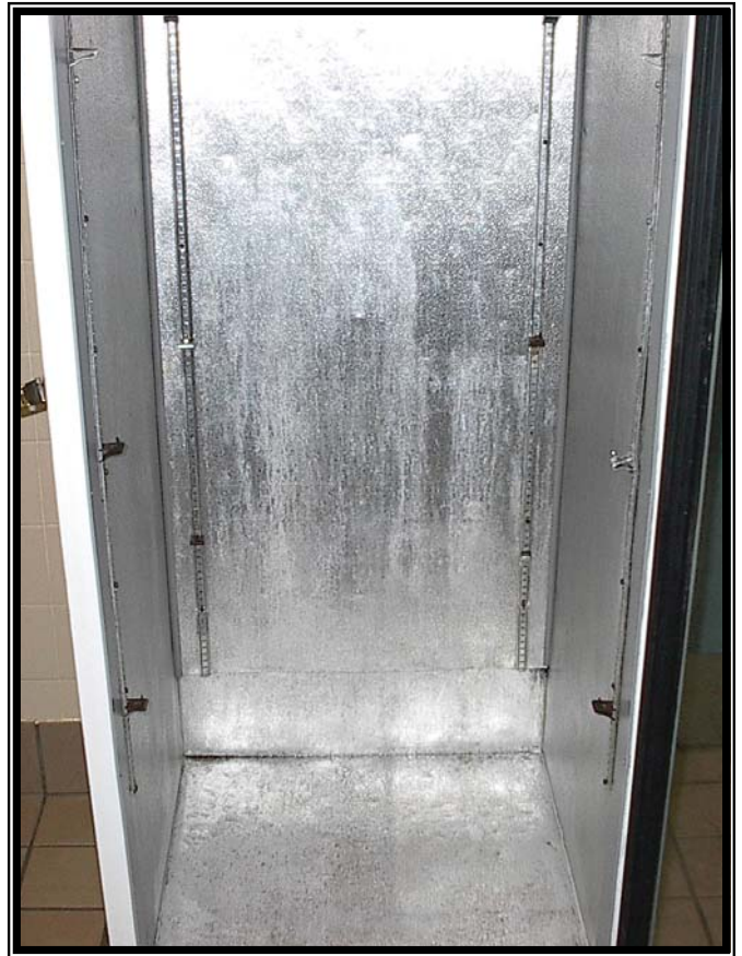
Display cases and collars are easily cleaned and sanitized using lance, brush, squeegee and/or suction tools.
